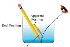
The ratio of the change in the speed of light is called the refractive index, and instrument that measure it is called refractometer. The refractive index of a liquid is related to its concentration and so a refractometer can display the concentration in suitable units, such as °Brix (sucrose), glucose, etc
